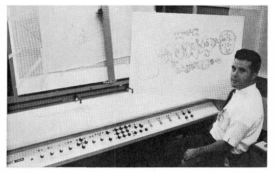
ILLUSTROMAT 1100 is operated by Ray Chavez of Technical Art Division 3463. The analog computing machine produces three dimensional perspective drawings when the stylus arms trace front and side views from an engineering blueprint. The drawing at right is an "exploded" view of an interval timer produced by the machine and inked for reproduction.
